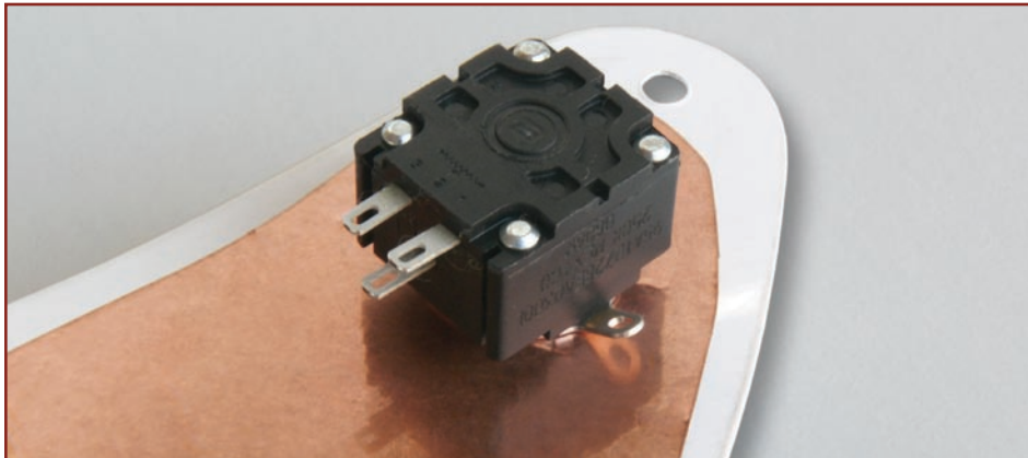
Figure 3: Correct mounting of solder lug lock washer
